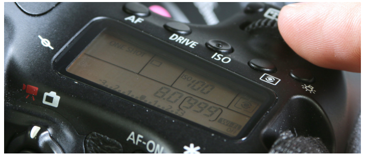
Fig 5 - Set Aperture to 8.0
