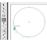
place second anchor 4) Place a second anchor point on the same line path, approximately 1/32th of an inch away from the first anchor. **Note:** 1/32" is the minimum line break width needed to keep objects attached to the original sheet material. To assist with estimating 1/32" line breaks, go to Preferences, Grid menu and change the Vertical and Horizontal Document Grids into a Gridline Every 1 inch with 32 Subdivisions.
